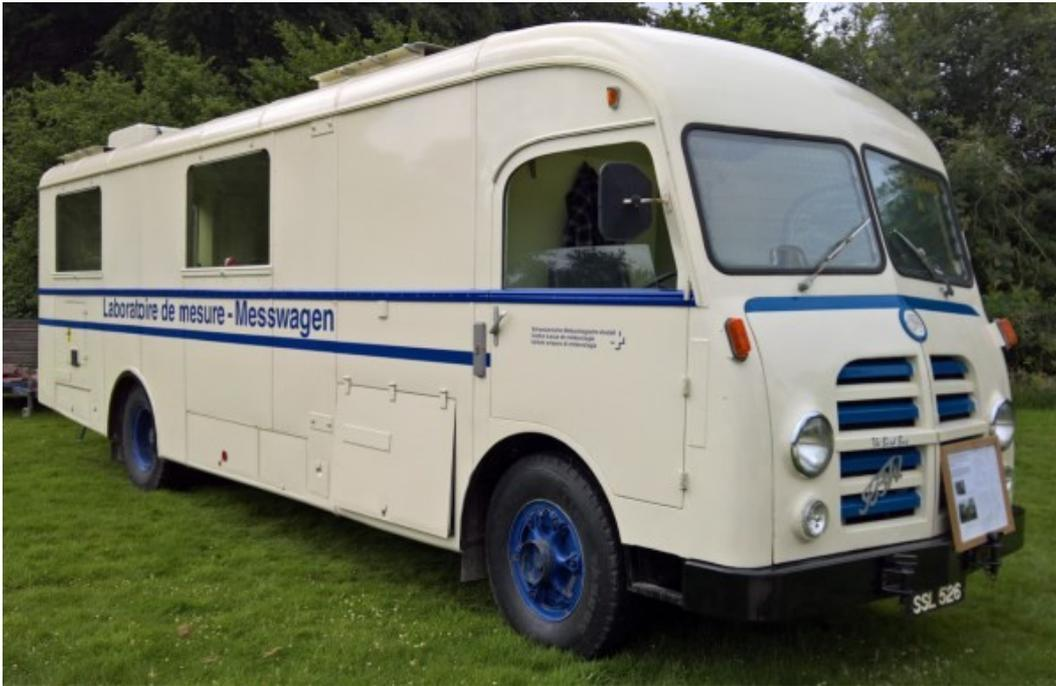
This example, owned by a local collector of what he called “his toys”, was built in 1954, initially for the Swiss Army as a mobile X-ray clinic able to travel to avalanche sites and the like. It has a six cylinder, 8.6 litre diesel engine, giving around 115 bhp and a comfortable maximum speed of 40 mph, though with the ability to climb as well, if a little slowly. Some one asked if it would do 70 mph, downhill? A brave idea, I suggest.
